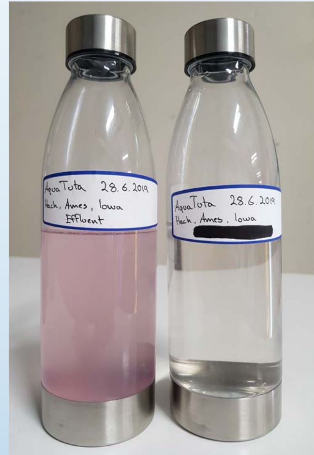
Example of heavy metal effluent treated with Aqua Tuta Left: Treated. Right: Untreated containing for example molybdenum and mercury
