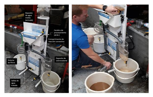
[Waste water deposit (input), Processing brain (at the back), Convective reaction compartment, Filter system, Supernatant deposit, Treated water output.]
