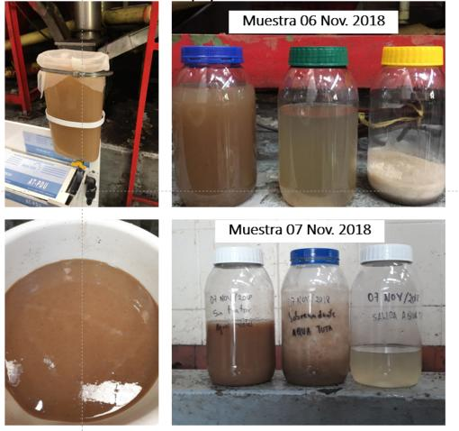
[Operation and output view for water treated with the PDU device, Sample Nov. 06, 2018, Sample Nov. 07, 2018.]
